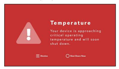
• A <u>thermal shutdown</u> notification presents onscreen if the battery temperature of 55°C (131°F) is reached or exceeded; at this time the Full Swing KIT automatically performs a thermal shutdown. To resume use of the Full Swing KIT following a thermal shutdown, turn the Full Swing KIT off, move it to a cooler environment, and keep it turned off until the Full Swing KIT has cooled down to normal use temperatures.
